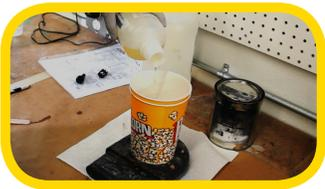
Very important to follow resin manufacturers instructions for proper measurements and mixing.
