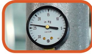
Epoxy resin run full vacuum at 20 to 24 in/HG until everything is saturated and cured.
