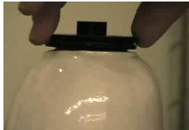
3. Carefully glue Integrator™ to mold and PVA bag.
