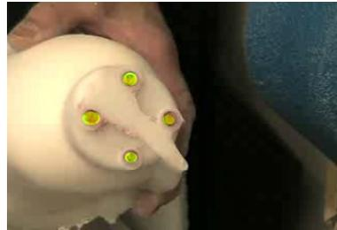
When plastic has cooled, expose foam dots, and grind the bottom of the socket as flat as possible without damaging posts
