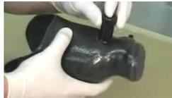
**21. Carefully thread valve body into valve base. Using lock wrench tighten to hand tight.**
