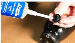
8. Run a small bead of Coyote Quick Adhesive around the edge of the valve base.
