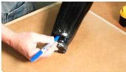
1. Mark the valve body location as close to the distal end of the socket as possible.
