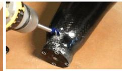
5. Drill a 1/2" for the valve body hole.
