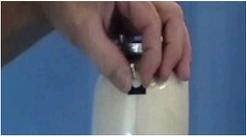
**14. Mark valve location on inner PVA bag and cover mark with tape to prevent tearing.**
