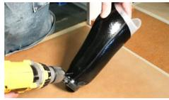
3. Use an 1/8" drill bit for pilot hole. Have flexible insert in socket when drilling pilot hole.
