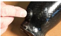
9. Carefully place the valve base in drilled hole. Hold base firmly in place.
