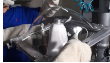
Pull preferred flexible plastic over socket and installed fabrication dummy using a vacuum system.
