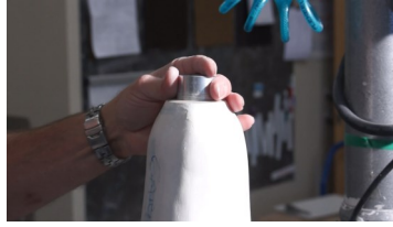
Pull preferred flexible plastic over socket and installed fabrication dummy using a vacuum system.
