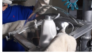
Pull preferred flexible plastic over socket and installed fabrication dummy using a vacuum system.
