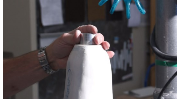
Pull preferred flexible plastic over socket and installed fabrication dummy using a vacuum system.
