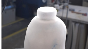
Let plastic cool before cutting fabrication dummy free.
