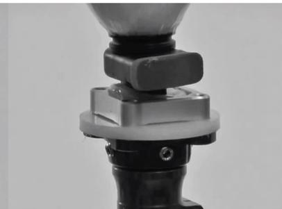
1. Place glue plate on connector. Install pyramid to connector. Do not over tighten screws.
