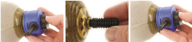
Install pin on liner. Engage lock to check for play between lock and liner.
